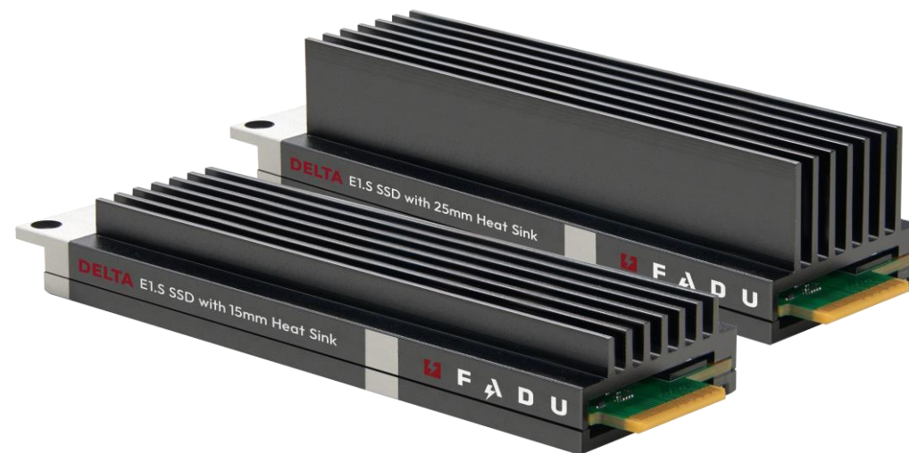
E1.S 15mm, 25mm Heat Sinks
